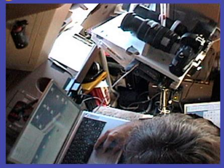
Cabling was rigged vertically downward and supported from below from platform center of gravity to minimize unbalanced torques on the platform.
