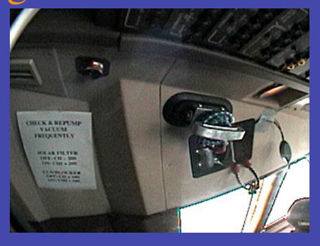
The camera platform was suspended from a bungie cord attached to a 70-lb static load capacity vacuum suction cup secured to the flight deck wall in a panel pass-through.
