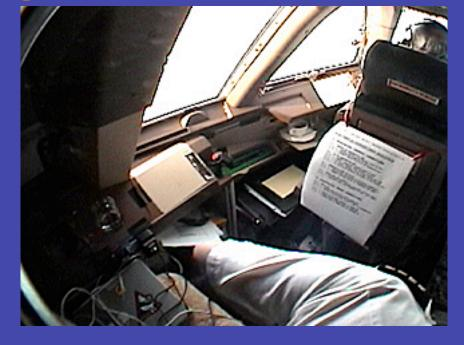
A sign hung right above the second observer's seat was a constant reminder to "check and re-pump" the suction cup vacuum pressure frequently.
