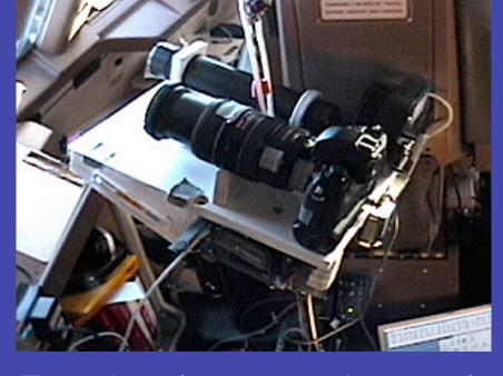
Camera/gyro platform fully rigged and suspended from flight deck wall, in position at observer's window behind pilot's seat ready for final balance and alignment check.
