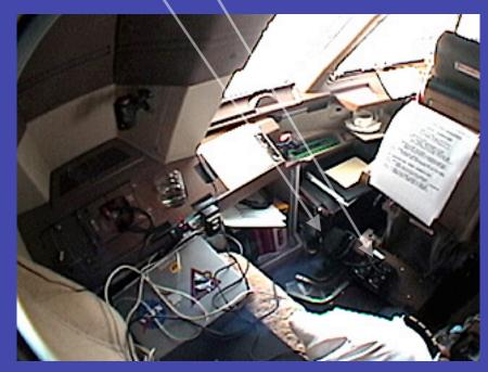
110 VAC 400 Hz gyro power inverters and Ni-Cad battery packs attached with velcro to bottom of pilot's seat and flight deck floor next to seat rail system.
